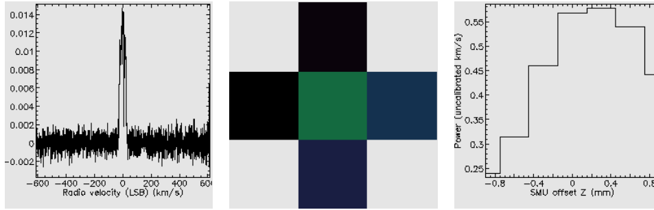
Figure 3. Preview images created by the ORAC-DR “summit” pipeline for heterodyne instruments. Left : a representative spectrum from a pointing observation. Center : a map showing the 5-point pattern used for pointing observations. Right : a graph showing the result of adjusting the position of the secondary mirror (SMU) in a focus observation.
